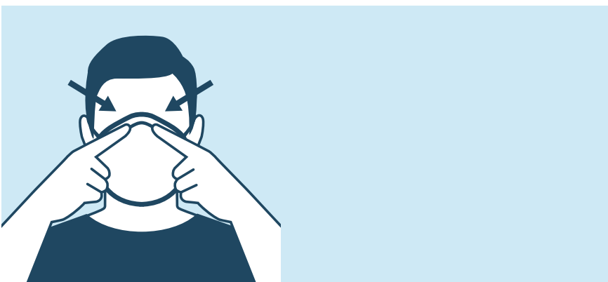
Use both hands to mold the nosepiece over the bridge of your nose; do not pinch the nosepiece
