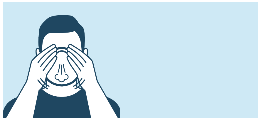
Perform a seal check: place hands over the respirator, exhale sharply, if air is felt on your face readjust respirator as needed and perform seal check again. When the respirator is a good fit, you will not feel any air on your face.
