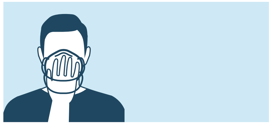
Place the N95 respirator on your face, covering nose and under your chin
